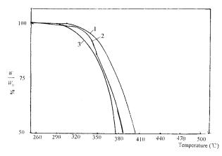
**Figure 4** Three TG scans of 3 different copolymers: (1)  $334^{\circ}$ C; (2)  $330^{\circ}$ C; (3)  $324^{\circ}$ C. *W* is the residual weight of the sample;  $W_{o}$  is the original weight of the sample.
