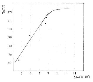
**Figure 5** Effect of  $M_w$ s on  $T_g$  values of heat-resistant PMMA (CHMI content: 10%).
