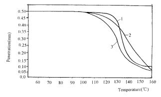
**Figure 3** TMA curves of 3 different copolymers: (1) 124°C; (2) 118°C; (3) 106°C.
